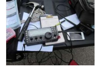
small lengths of coax and a couple wire antennas that fits in a small camera bag. Though the radio has batteries I brought a 7 Ah gel cell for power.
