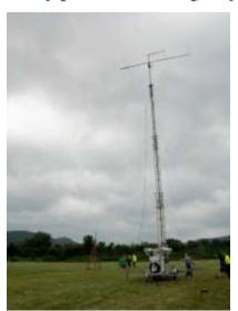
integrated feed lines the three piece nested aluminum structure will quickly place antennas at 50 feet.
