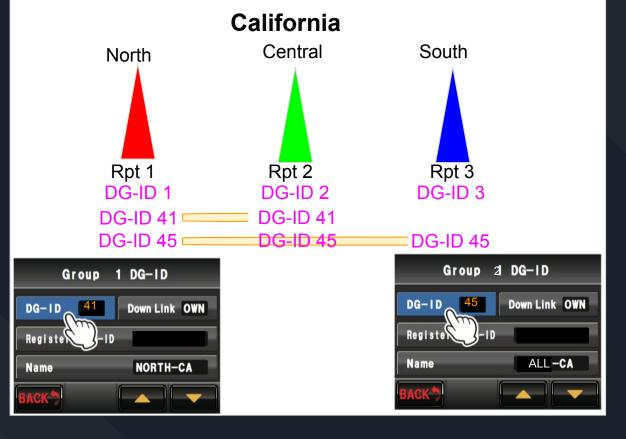
Once HH 3 keys up (and no repeaters had an active TOT,) all the repeater TOT will start, and ALL repeaters will be transmitting. (HH 3 will hear a Single Beep indicating the TOT started.)
