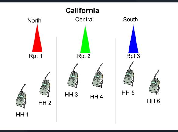
HH 1 and HH 2 select DGID TX-01 in their radios. When they transmit, Rpt 1 works like a normal repeater.
