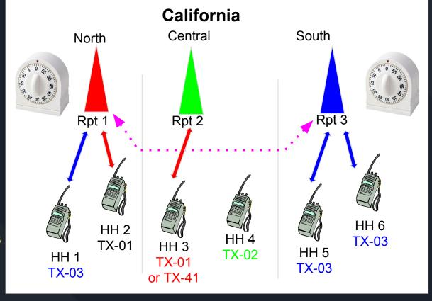
{ Once a Repeater to Repeater link is made and timers are running, other repeaters are locked out }
